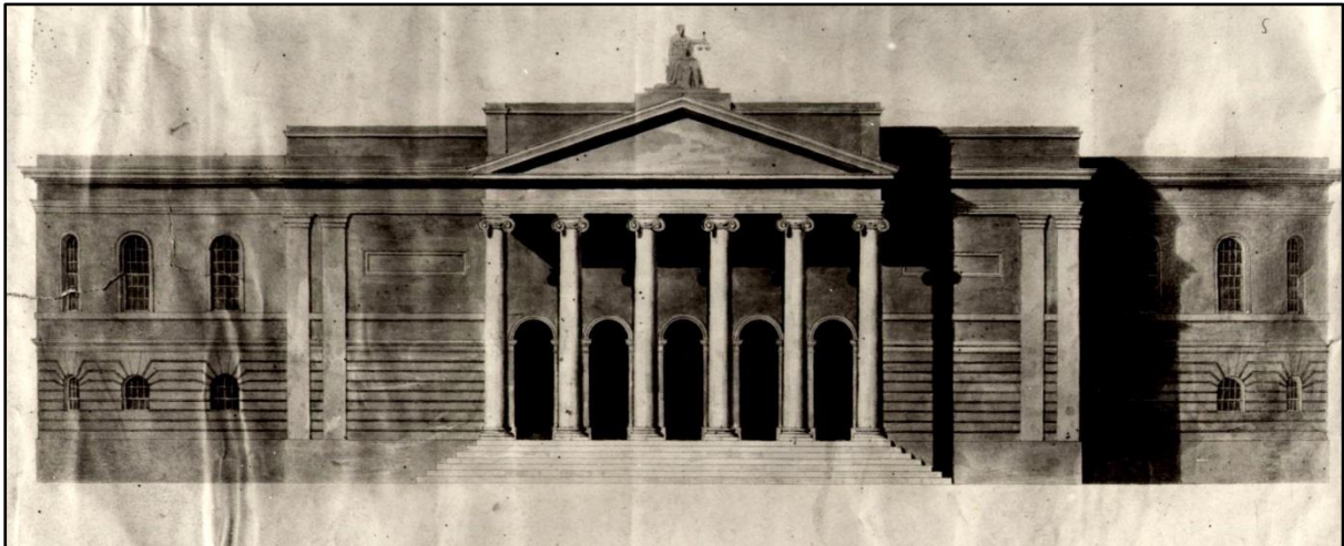
Fig. 11. Tullamore courthouse, front-elevation drawing, unexecuted. John B. Keane, c. 1833. In this scheme the courtrooms would have dictated the semi-circular form of the wings, but for unknown reasons this design was later altered to make it more like G.R. Pain's plan for Cork (see Chapter 2). Reproduced courtesy of Michael Byrne.
